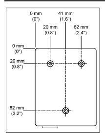
Each IS6520/MS6520 Cubit<sup>®</sup> is equipped with three threaded mounting holes located on the back of the scanner. The following diagram shows the exact location of each mounting hole. The mounting holes are 6 millimeters deep and are threaded for use with 3 millimeter screws.
